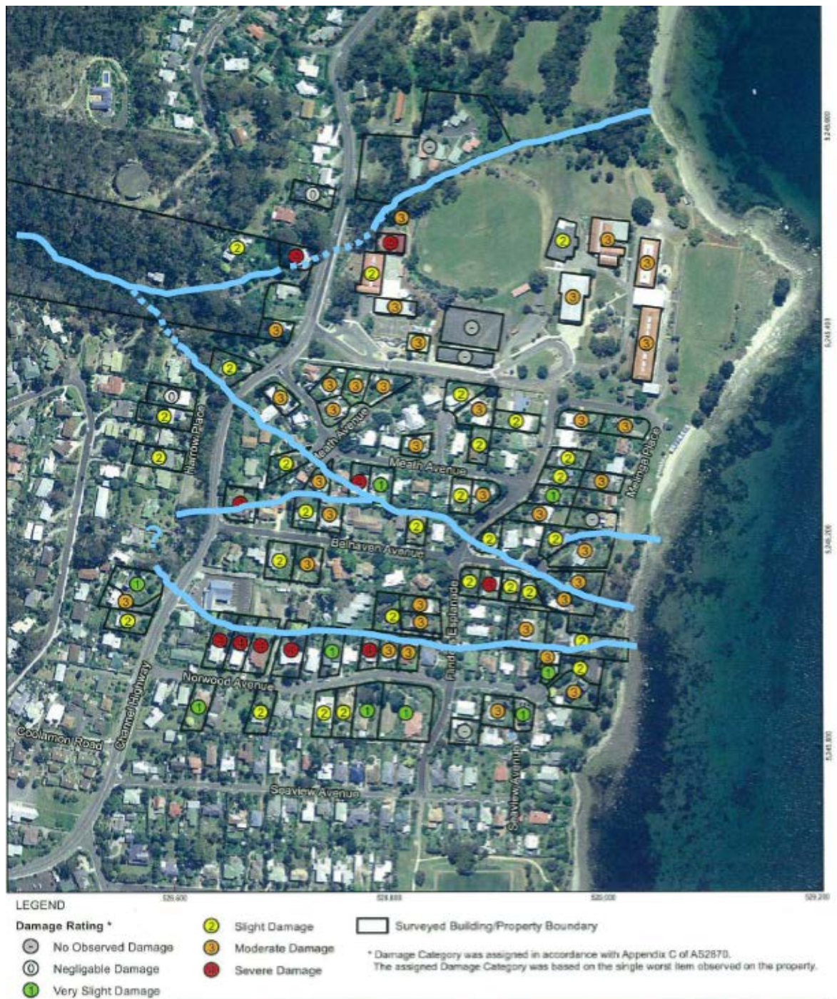
Figure 4 Plan showing overlay of building damage survey results and infilled stream locations
