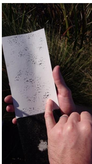
Rat tracking tunnels baited with peanut butter and an example of the rat tracks recorded
