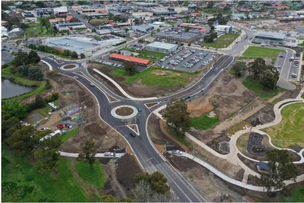
Figure 4 – New Goshawk Way extension including roundabout, pedestrian underpass and upgraded John St roundabout - October 2022.
