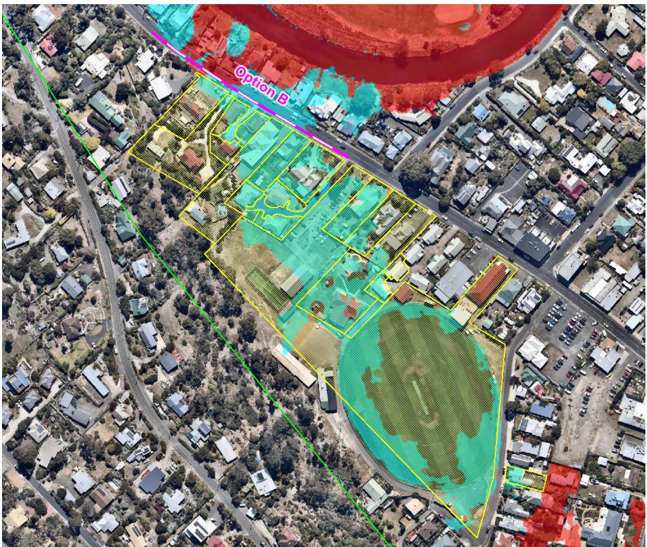
Diagram 6: Properties (highlighted in yellow hatches) Protected by Option B under Year 2100 Climate Condition.
