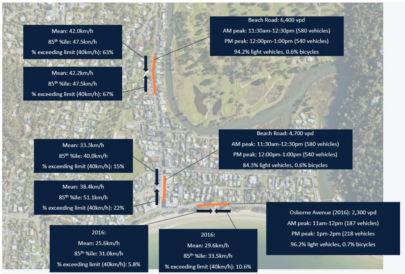
Figure 9: Overall Summary of Key Traffic Survey Data
