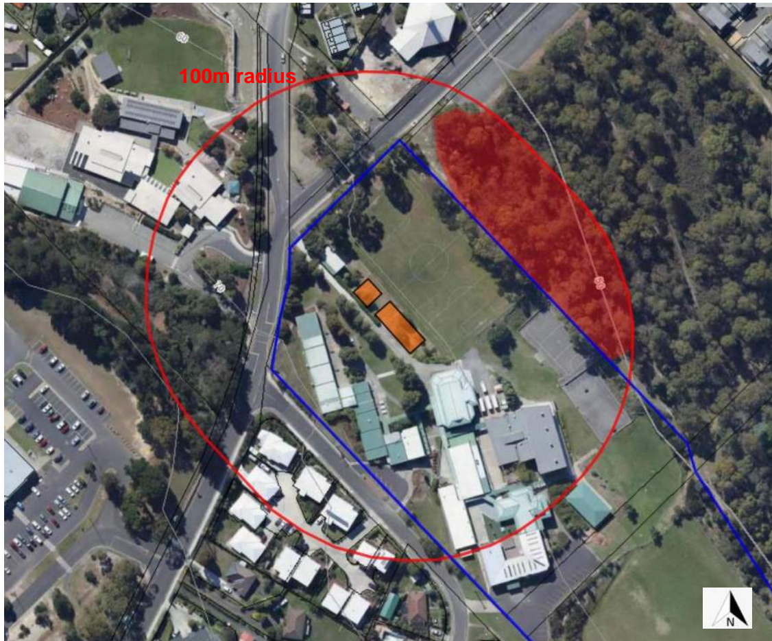
Figure 4: contoured TasVeg4.0 listmap. www.thelist.tas.gov.au Property outline in blue, proposed classrooms in orange. Red shading indicates down-slope bushfire prone woodland vegetation within 100m of proposal, approximately 55m from the site.
