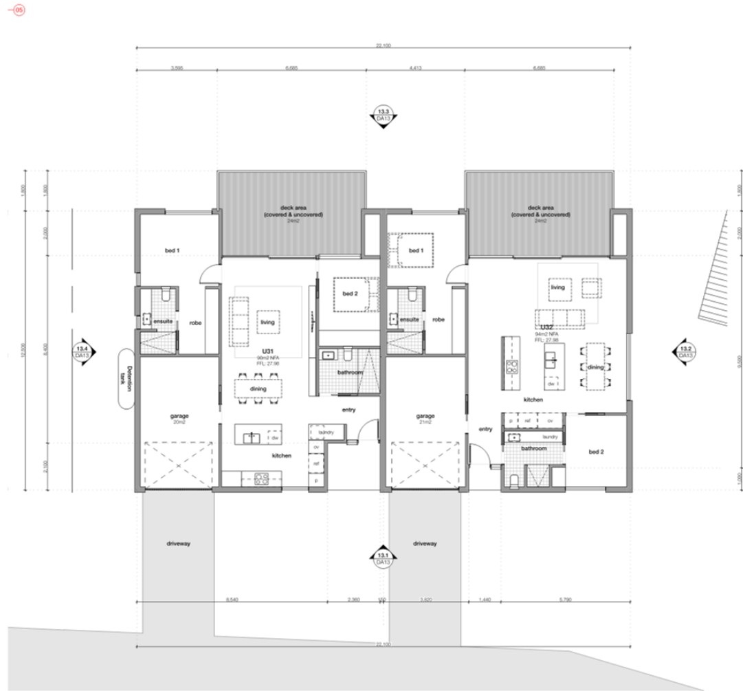
1. Typical Duplex Plan (U31-U32) Scale 1:100
