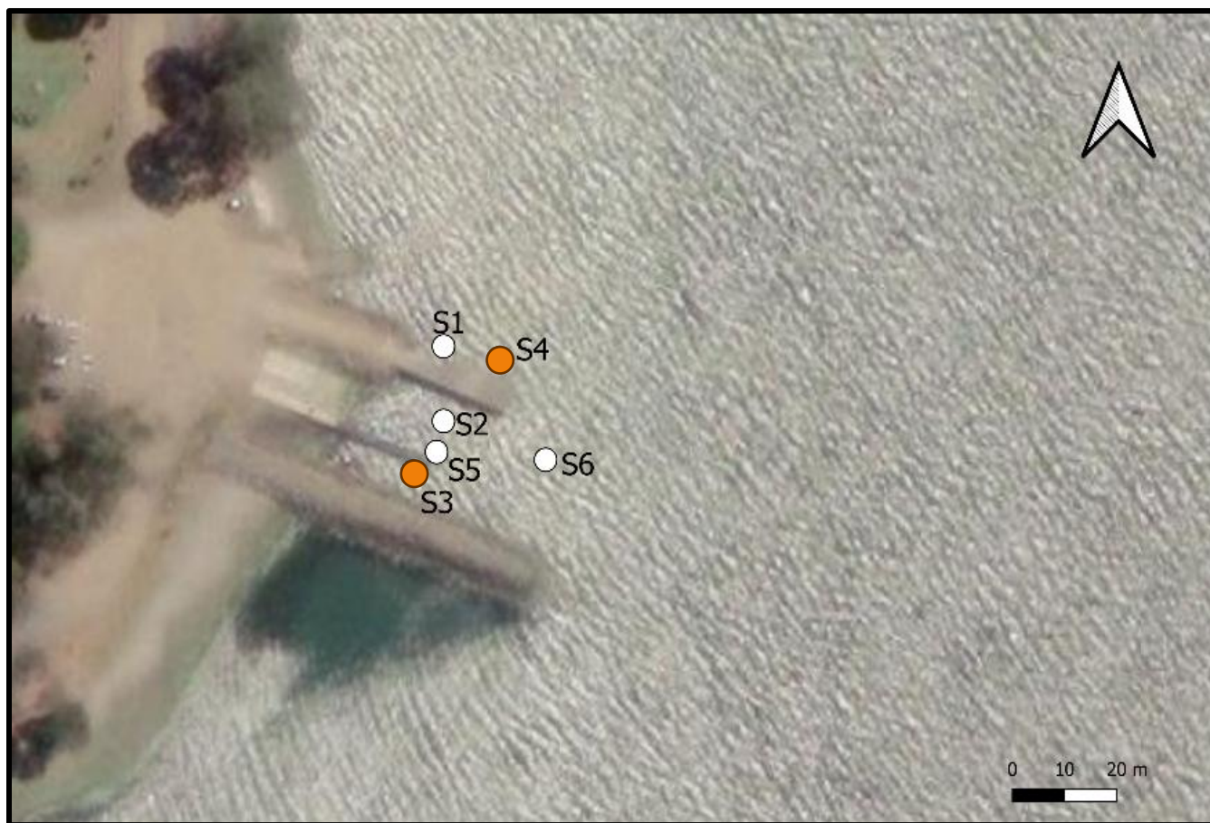
Figure 8. Locations of sediment samples extracted for laboratory testing. One sample for particle size analysis and contamination were taken from each site. S3 and S4 (orange points) were collected using a vibrocorer. ASS/PASS testing samples were taken at S1 and S2. Sediment settling tests were conducted using sediment collected at S3, S4, S5 and S6.
